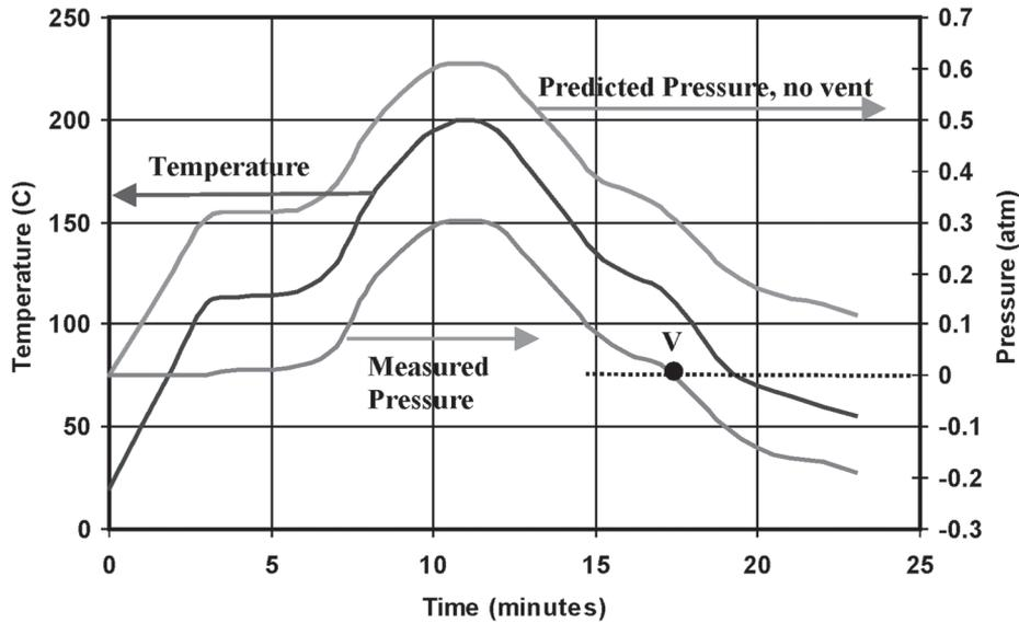
Fig. 9 Measured mould pressure for a warped part
