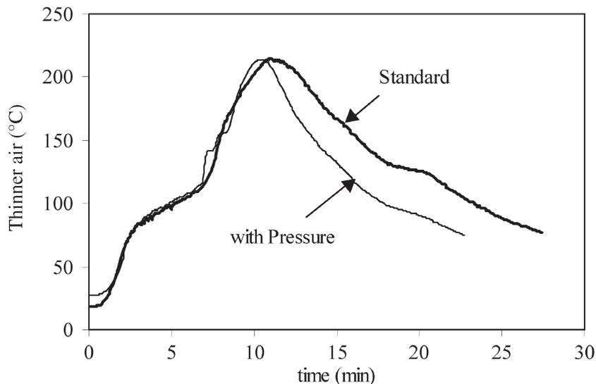
**Fig. 5** Rotolog traces of polyethylene mouldings with and without pressure
