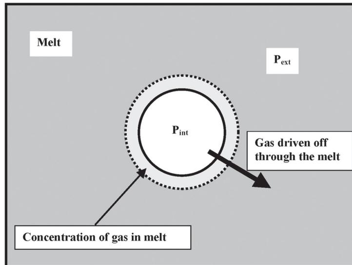
Fig. 1 Mechanism by which bubbles disappear from the melt
