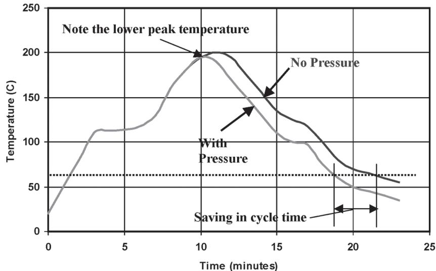
Fig. 2 Rotolog traces of polyethylene mouldings with and without pressure
